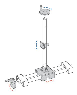
Combined single and double tube linear units with moving in X and Z direction
