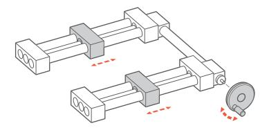
Multi-axis systems with adjustment in X direction
